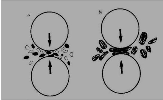
**Fig.1. Fracture- welding mechanism during powders milling.**
