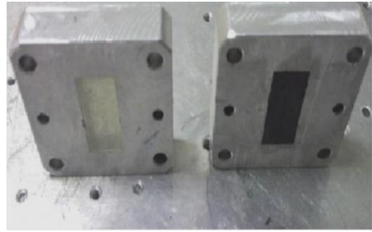
**Fig.2. Nanocomposite sample within Rectangular Waveguide.**
