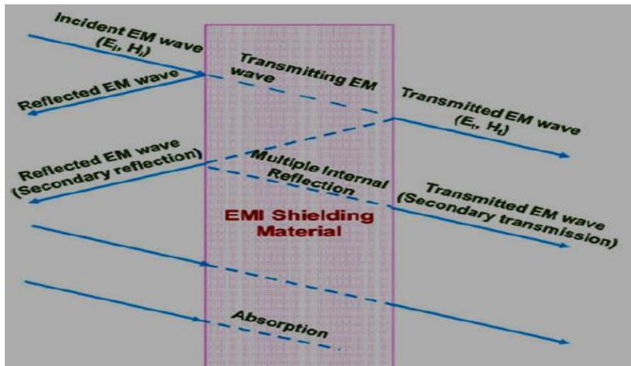
The absorption factor is a microwave parameter calculated using the squared scattering parameters  $S_{11}$  and  $S_{21}$ :
