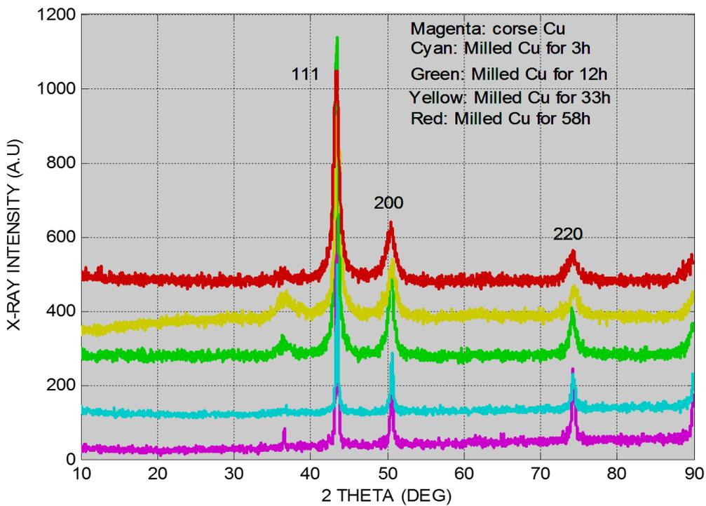
**Fig.3. XRD Spectra of coarse and milled Cu powders.**
