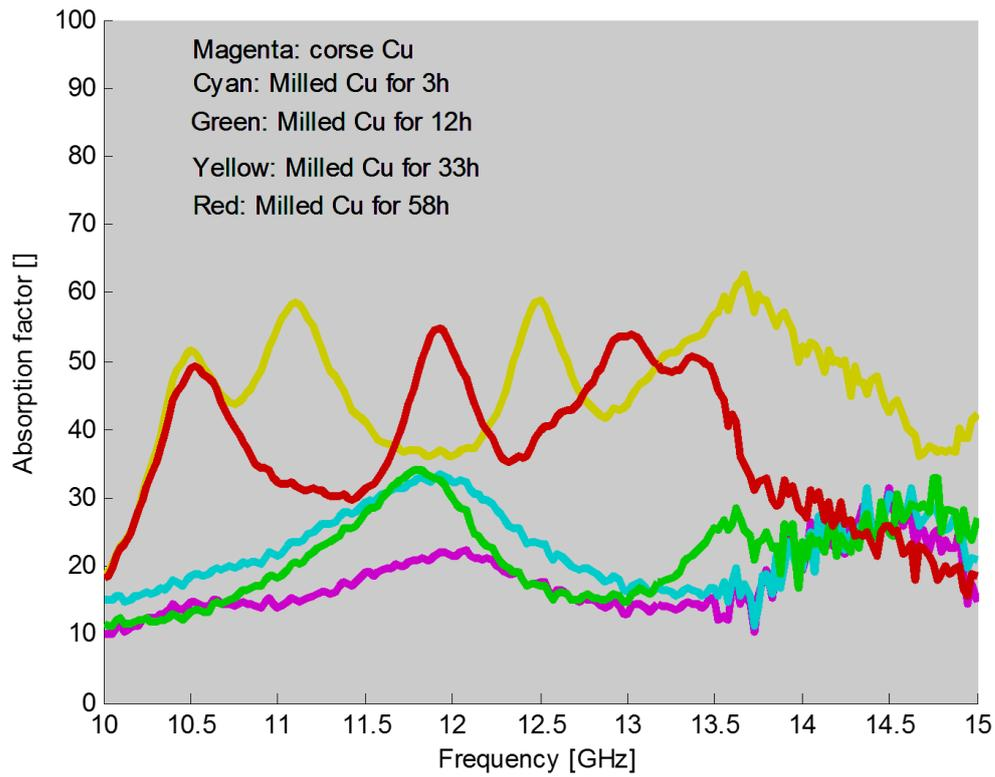
The computation of complex dielectric permittivity followed the noniterative approach proposed by A.H. Boughriet. Dielectric permittivity spectra exhibit the effect of the structural refinement and the resulting morphology on the microwave absorbing properties.
